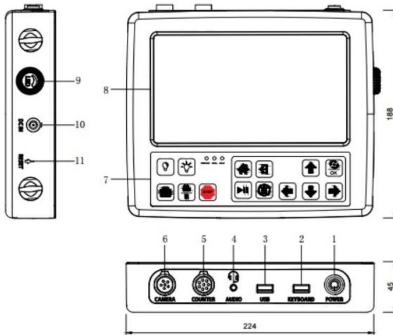
1. POWER Press the button for 3 seconds to turn on /off the control box
